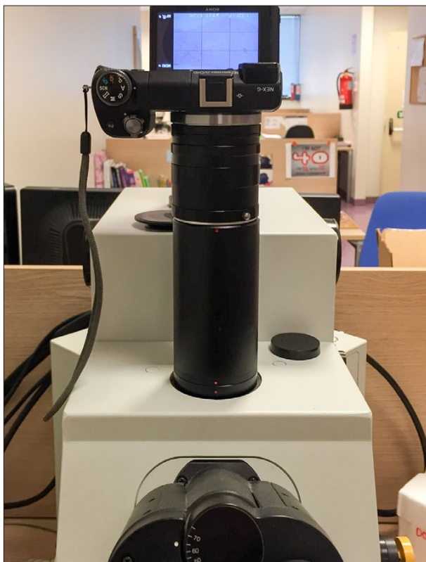
"Figure 1 - video acquisition setup"
